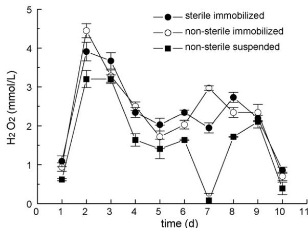
**Fig. 5.** H<sub>2</sub>O<sub>2</sub> excreted by *P. chrysosporium* under different conditions: (●) immobilized with polyurethane foam under sterile condition; (○) immobilized with polyurethane foam under non-sterile condition; (■) suspended under non-sterile condition.
