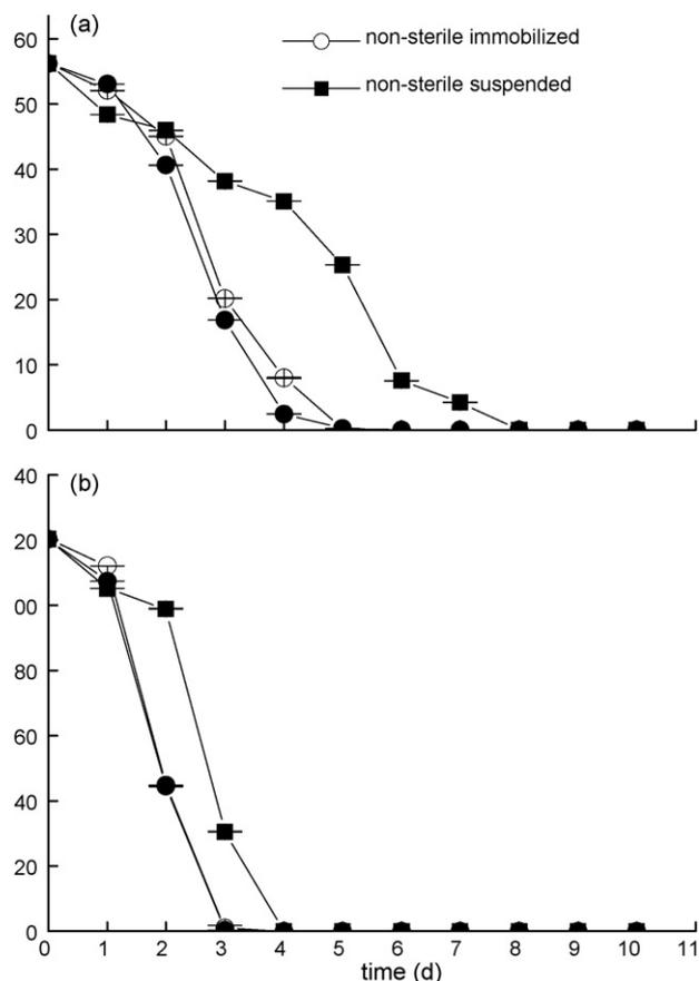
**Fig. 4.** Nutrient consumption by *P. chrysosporium* under different conditions: (●) immobilized with polyurethane foam under sterile condition; (○) immobilized with polyurethane foam under non-sterile condition; (■) suspended under non-sterile condition.
