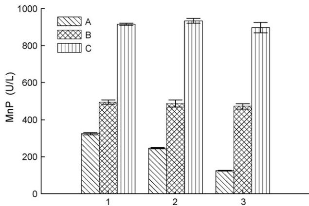
**Fig. 1.** MnP excreted by white rot fungi of suspended (A) and best immobilized culture with reticulation (B) and polyurethane foam (C). 1, decolorization under sterile condition after incubation under sterile condition; 2, decolorization under non-sterile condition after incubation under sterile condition; 3, decolorization under non-sterile condition after incubation under non-sterile condition.
