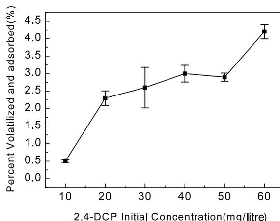
Fig. 2. Abiotic loss of 2,4-DCP at various initial concentrations in the reactor.
