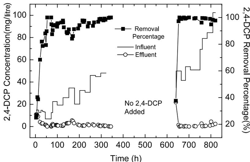
Fig. 7. Continuous biodegradation of 2,4-DCP.
