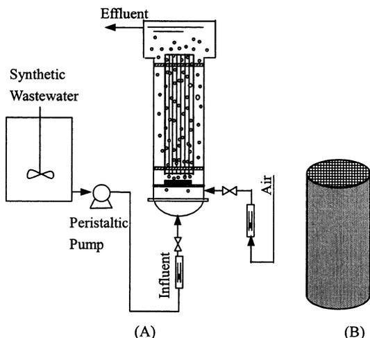
Fig. 1. Schematic diagram of the novel bioreactor (A) and the profile of the honeycomb-like ceramic carrier (B).
