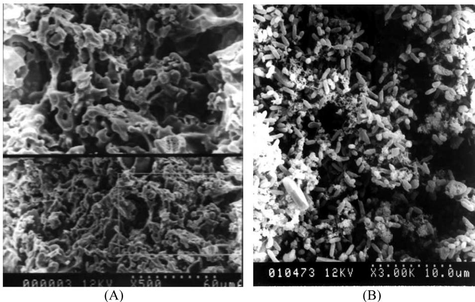
Fig. 3. Scanning electron micrograph of (A) Honeycomb-like ceramic carrier without microbes and (B) Honeycomb-like ceramic carrier immobilized with 2,4-DCP-degrading microbes.
