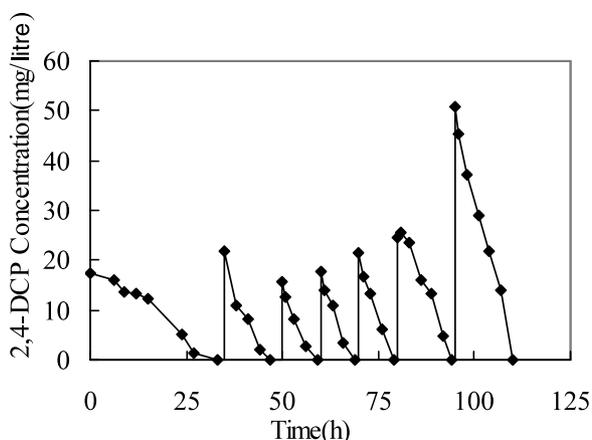
Fig. 4. 2,4-DCP degradation as a single substrate in the reactor operated in fed-batch mode.
