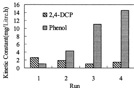
Fig. 6. The variation of rate constants for the biodegradation of phenol and 2,4-DCP.
