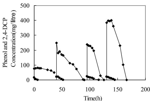
Fig. 5. Biodegradation of 2,4-DCP using phenol as co-substrate (◆) phenol concentration, (●) 2,4-DCP concentration.
